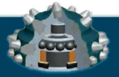
Standard bit bearings are assembled with O-section elastomeric seals (RS), bushings and washers are of maximum sizes. This allows to high axial drilling loads on the bit to obtain maximum ROP rates when drilling hard rocks.
