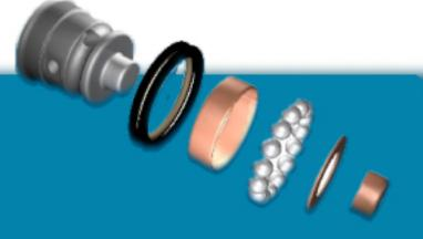
The bushings and washers are coated with a layer of wear-resistant alloy, and the mating surfaces of the cone body are silver coated, which greatly increases the load capacity of the bearing.
